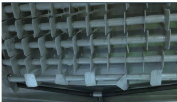
11. Cut off the original heater drain clip, and then install the new one. Make sure the new clip is wrapped securely around the heater and that the tail portion does not touch the plastic liner.
