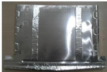
9. Carefully reinstall the evaporator and drain plate. Make sure they are securely positioned.
