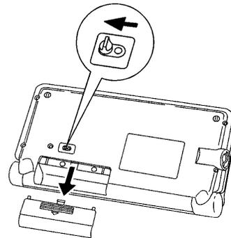
3. Insert two batteries on top of the ribbon tab, making sure they are positioned correctly according to plus (+) and minus (-) polarity, as shown below.
