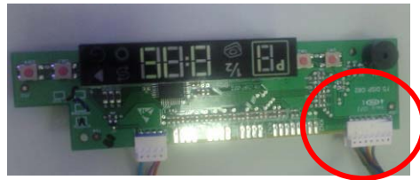
DISPLAY BOARD : KN1 connector
