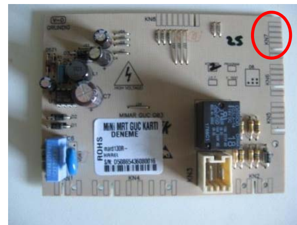
POWER BOARD: KN7 CONNECTOR
