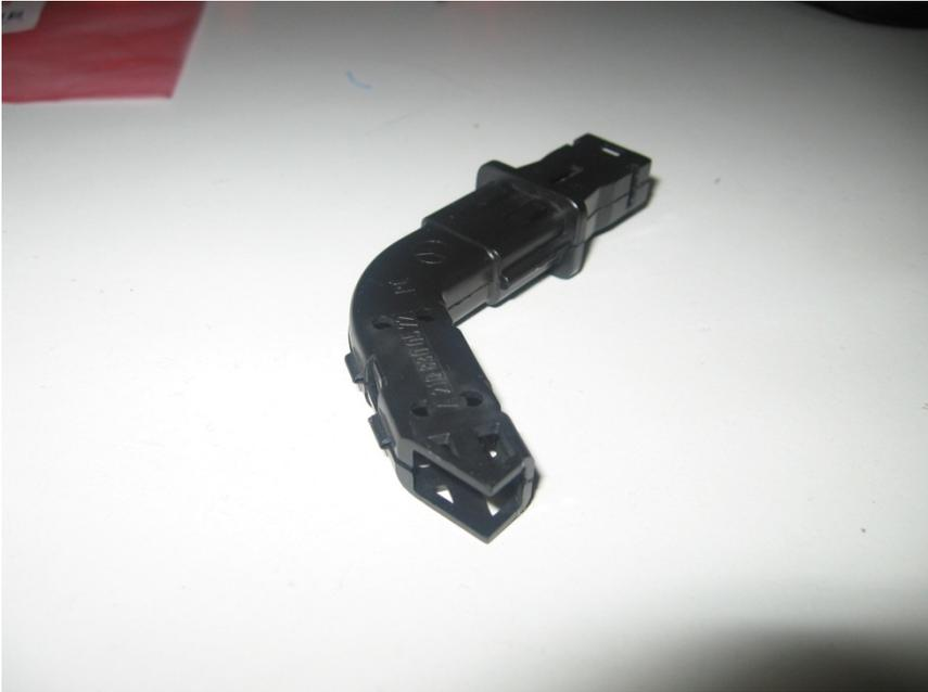
If you operate the climate control (heater or A/C) without evaporator temperature probe on its place, a trouble code may be thrown. You have to clear it after installation of the sensor.
