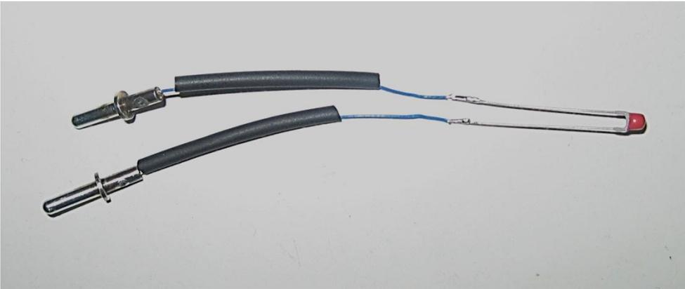
Install whole assembly into its plastic case. There are two thin passages in red circled area, install blue cables into those passages to not squeeze them after the closure of the case.
