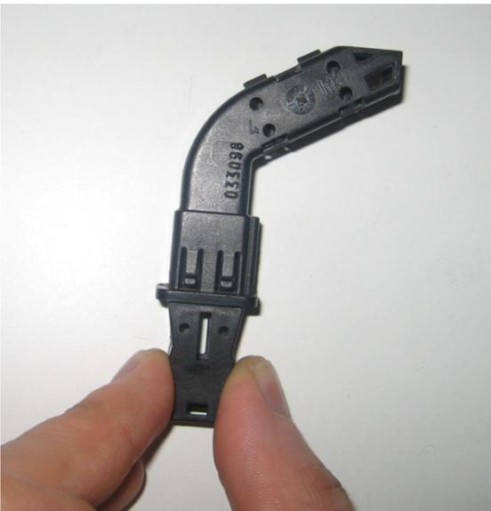
There are two notches in front part of the sensor (you can see them in red circles on the following picture) you have to release them first, but the rear part is glued. You need to separate two halves of the sensor by cracking glue with the aid of a knife/flat head screwdriver etc.
