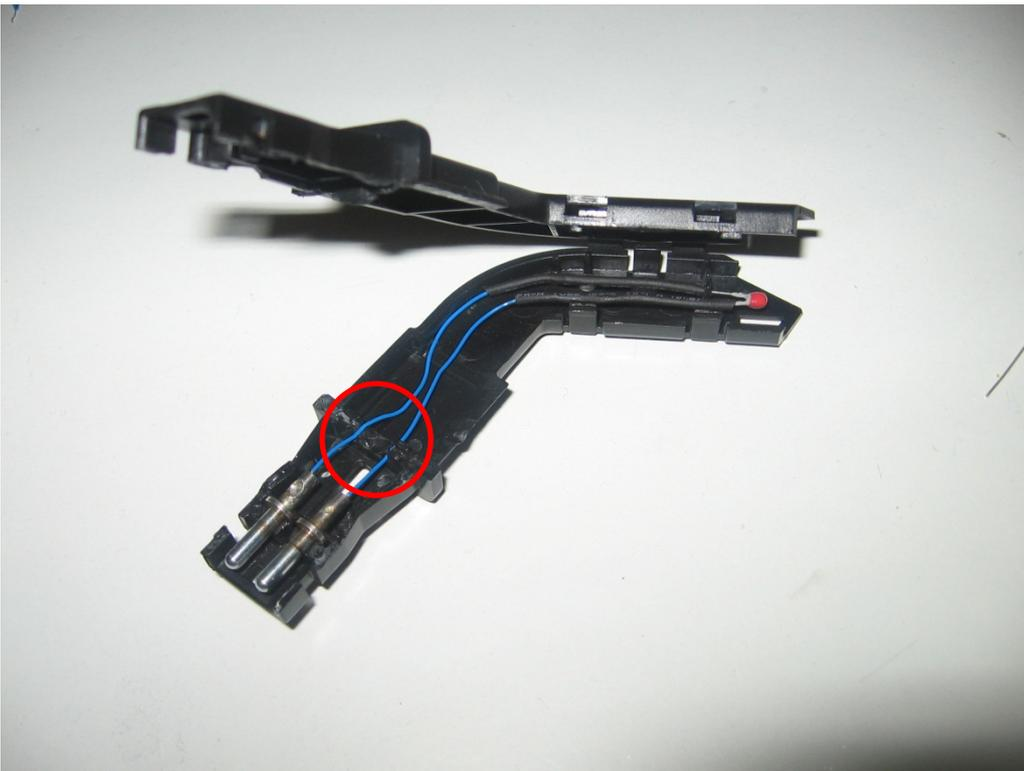
Put few drops of cyanoacrylate adhesive (Pattex etc.) to the originally glued part of the sensor and close the halves. Keep squeezing the back side for few minutes to guarantee the adhesion. After then, your sensor is ready for installation.
