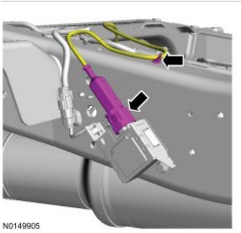
3. **NOTE:** If necessary, lubricate the NOx (Nitrogen Oxides) sensor with penetrating and lock lubricant to ease removal.
