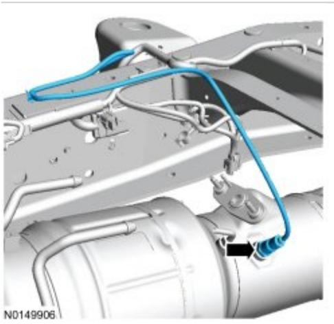
5. **NOTE:** Do not apply any type of electrical grease or lubricants to the electrical connector.
