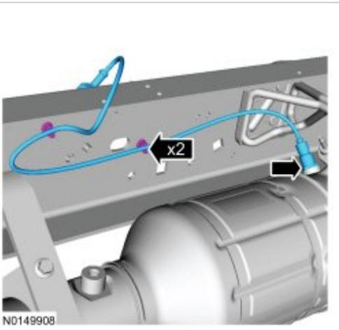
3. **NOTE:** Do not apply any type of electrical grease or lubricants to the electrical connector.
