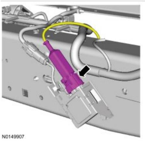
5. **NOTE:** If necessary, lubricate the NOx (Nitrogen Oxides) sensor with penetrating and lock lubricant to ease removal.
