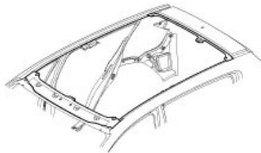
2. Clean the body bonding surface with a sponge dampened in alcohol. After cleaning, keep oil, grease and water from getting on the clean surface.
