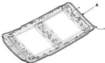
7. Fix the panorama roof to center hall (A) of body, install carefully the panorama roof to the body frame.
