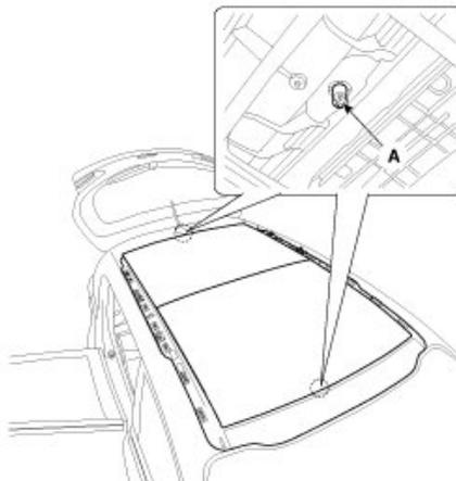
8. Check the Clearance and gap for each side after installing the panorama roof.
