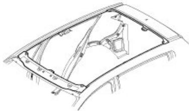
5. Apply a light coat of glass primer to the outside of the fasteners.
