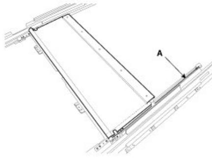
5. After loosening the roil blind mounting screws, and removing the rivet, remove the roil blind (A).
