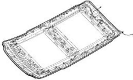
3. Remove front glass of the panorama roof by using a cutter knife.
