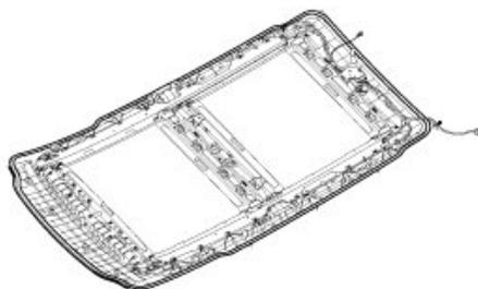
6. Pack adhesive into the cartridge without air pockets to ensure continuous delivery. Put the cartridge in a caulking gun, and run a bead of sealant (B) around the edge of the panorama roof (A) as shown. Apply the adhesive within 30 minutes after applying the glass primer. Make a slightly thicker bead at each corner.
